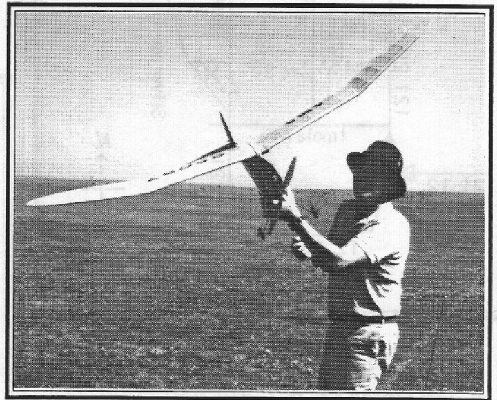
Don Bekins 72" Playboy, McCoy '49 power flies class C ignition, also set up for: class B ignition Torp 29, class B glow K&B 4.9cc, electric Texaco, electric LMR
