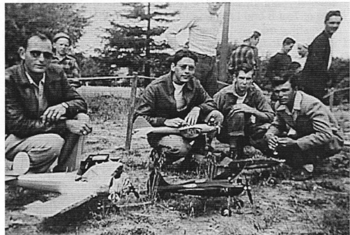
Nick's Whirlaway has a mono gear and fiberglass cowling, made in one piece. Still to be cutout for exhaust and controls. The wingspan is 81.5 inches and powered by an ORR 65. Nick plans on using the ship in LER. SAMSPAN covered.
