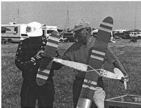
Jerry Rocha assists Bud Romak by lighting the dethermalizer fuse as Bud is wound and ready.
