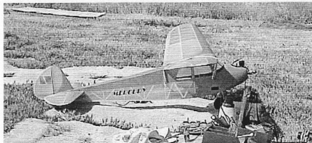
A nice side-view of the Mercury. Park constructed a very handsome cowling for the Ohlsson .60. Park printed his own decals.
