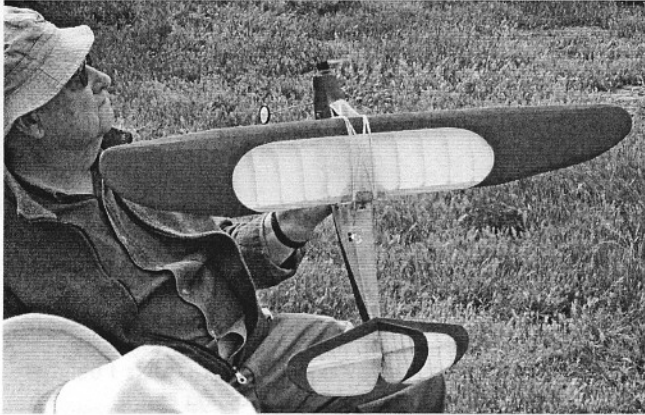
John Carlson admiring his electric Airborne. This ship is a good flyer and has a Jet Set M100 motor for power. It climbs at a good, even impressive, rate but John has plans to replace the motor with an M250 which is the same motor with different wiring.
