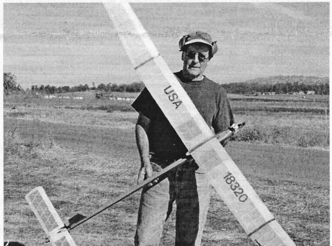
Paul Stauber with one of his hot free flight models - he double covers with Japanese tissue. Paul usually tests his models at the TOFFF sessions - fun to watch! The engine and timer installation is shown below - a squeeze-off. HOT!
