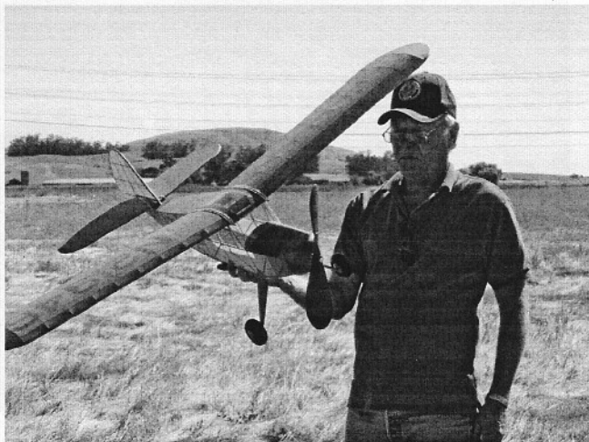
Gayle Wagner with his 54" scale-like rubber ship. Sixteen strands of 3/16" rubber, with a gross weight of 298 grams. Looks superb in flight doesn't it? An exciting project.
