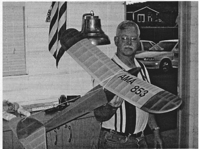
Bill Vanderbeek at Show and Tell with his latest old timer 1/2A RC Texaco ship. It is a Pixey, .049 power, 300 sq. in. A 1938 Schumacher design.
