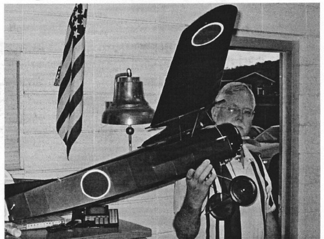
Bill Vanderbeek , below, hangs out with speedy builder Bud Romak and speedy building has rubbed off. Here is Bill's latest creation. The plane is our first free flight version of the Earl Stahl Fokker D-8. Power is an O&R .29 ignition engine. Color scheme is a Dutch version of the plane, samspan covering and dope finish.
