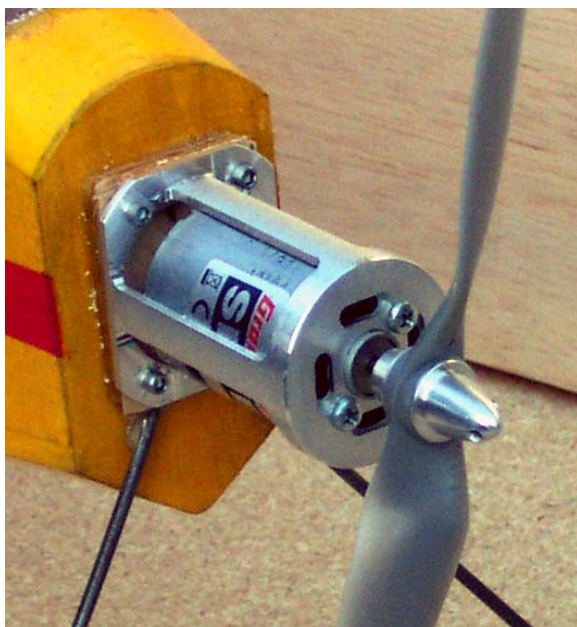
Loren Kramer's mount that can be used for 1/2a, speed 400, or an outrunner. It was designed by and is available from Loren Kramer at a very reasonable price.
