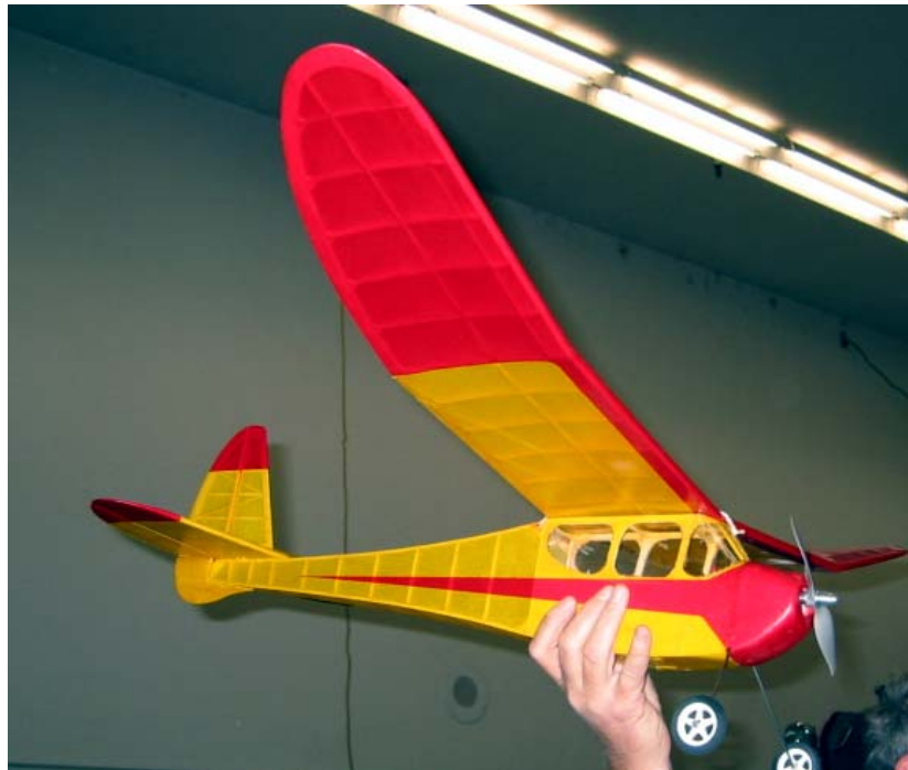
Loren Kramer's nicely done Cleveland Viking. From a set of original plans of 1940. Wingspan is 48" and 288 in 2 . This model is covered with polyspan and finished with Higgins ink and Design Master Paint for color. Flying weight is 14 oz. with an AXI 2208 brushless motor and 2 cell Li-Po battery.
