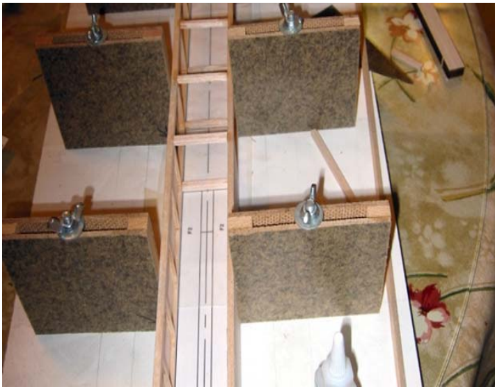
I have a nice fuselage jig for joining the sides; it's nice but not necessary.
