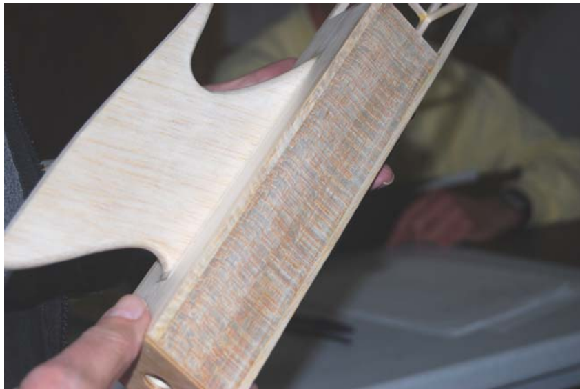
A Nice example of C-grain balsa used on the sides of a Kerswap.
