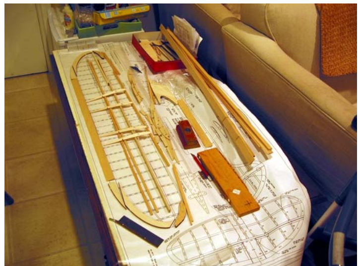
Layout the leading edge, tip parts, and trailing edge then add the ribs but not the spars. Glue this assembly together.
