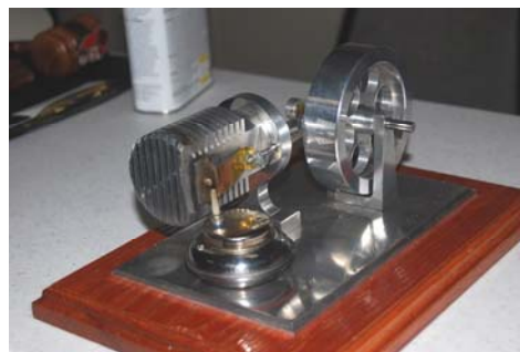
Ed Solenberger's finely machined external combustion engine.—very unique but very little power.
