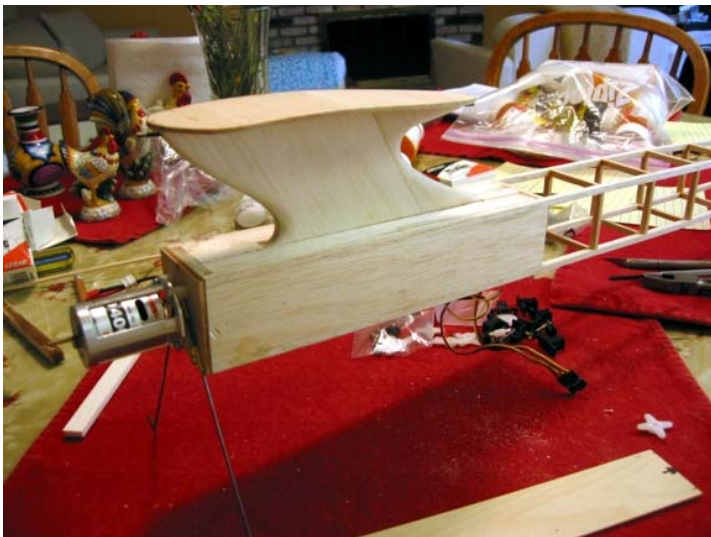
It's starting to look like an airplane now. Install everything else and temporarily hinge the rudder and elevator. You should have a complete airplane ready to finish.
