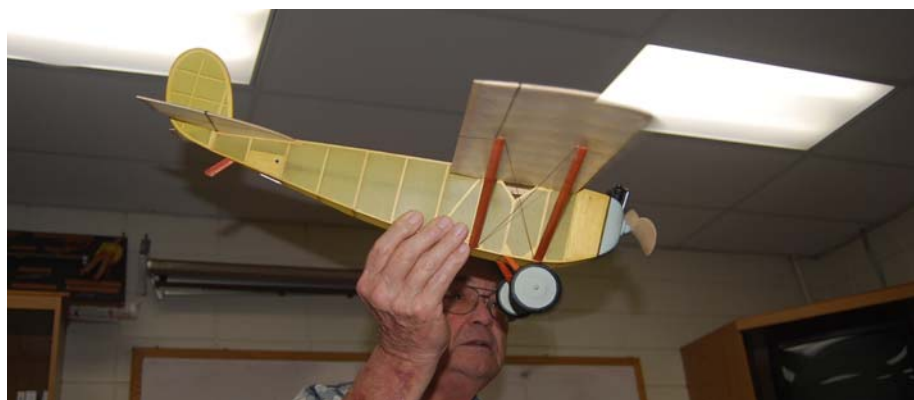
A Nice example of C-grain balsa used on the sides of a Kerswap.
