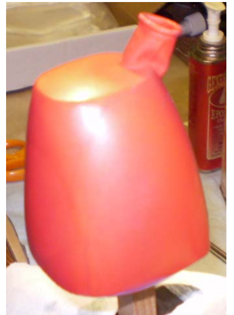
A balsa plug is made for the cowl and then a balloon is stretched over that
