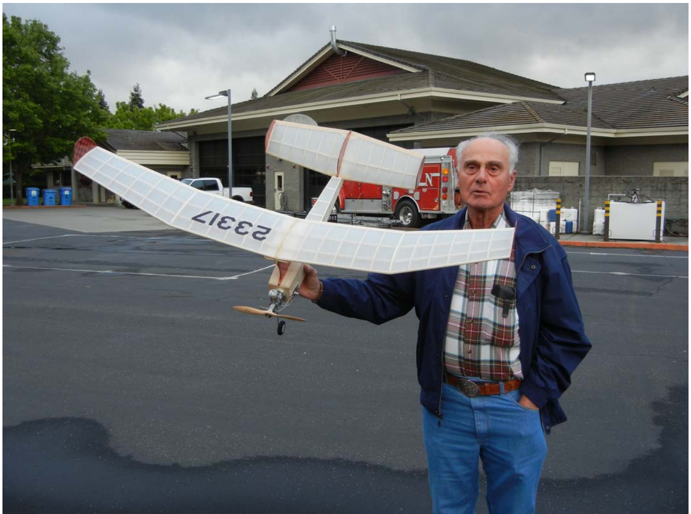
Jerry Rocha showed his free flight 52 inch Strato Streak powered by a .15 Elfin diesel replica, with a Texas timer for fuel shutoff and DT.
