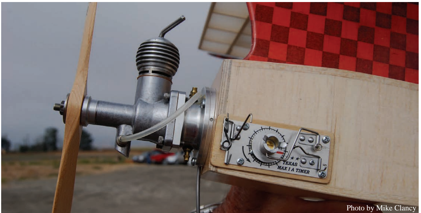
A closer view of Jerry's Strato Streak showing the timer and his custom engine mount with thrust adjusting plate for the diesel engine.
