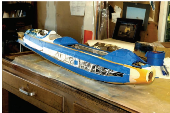
Picture #9 The fuselage masked for the black dope. Aluminum foil is the best mask.
