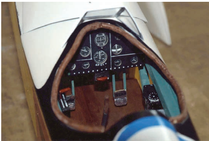
Picture #20 A close view within the cockpit. Note the rudder pedals
