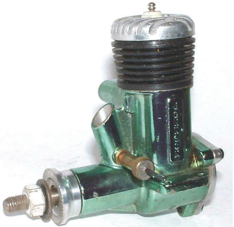
The green shade on the Johnson JBB-36 above reflects the metallic green paint job on the 35s. This is a carry over from the green anodized cases of the Orwicks which the engine resembled. This green factory painting only applied to the 35—not the lower displacement engines
