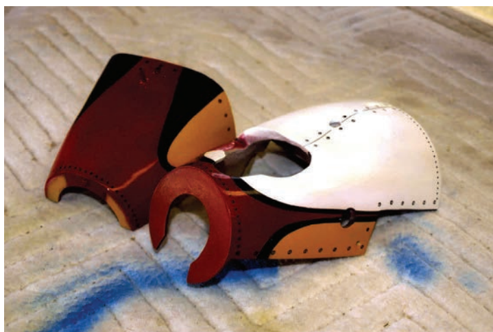
Picture #14 Note the rivets and dzus fasteners put on with a sharpie pen.
