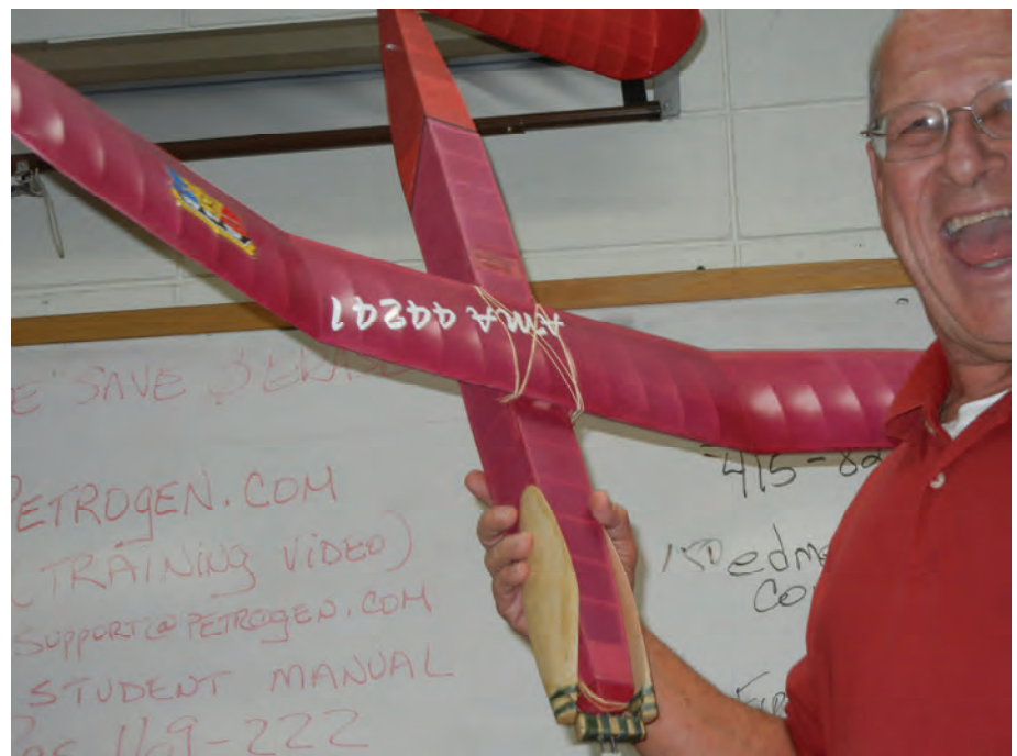
Rod Person's Red Buzzard. This was the commemorative model at the SAM champs this year. Rod's model has 14 loops of rubber that is wound 600 times.
