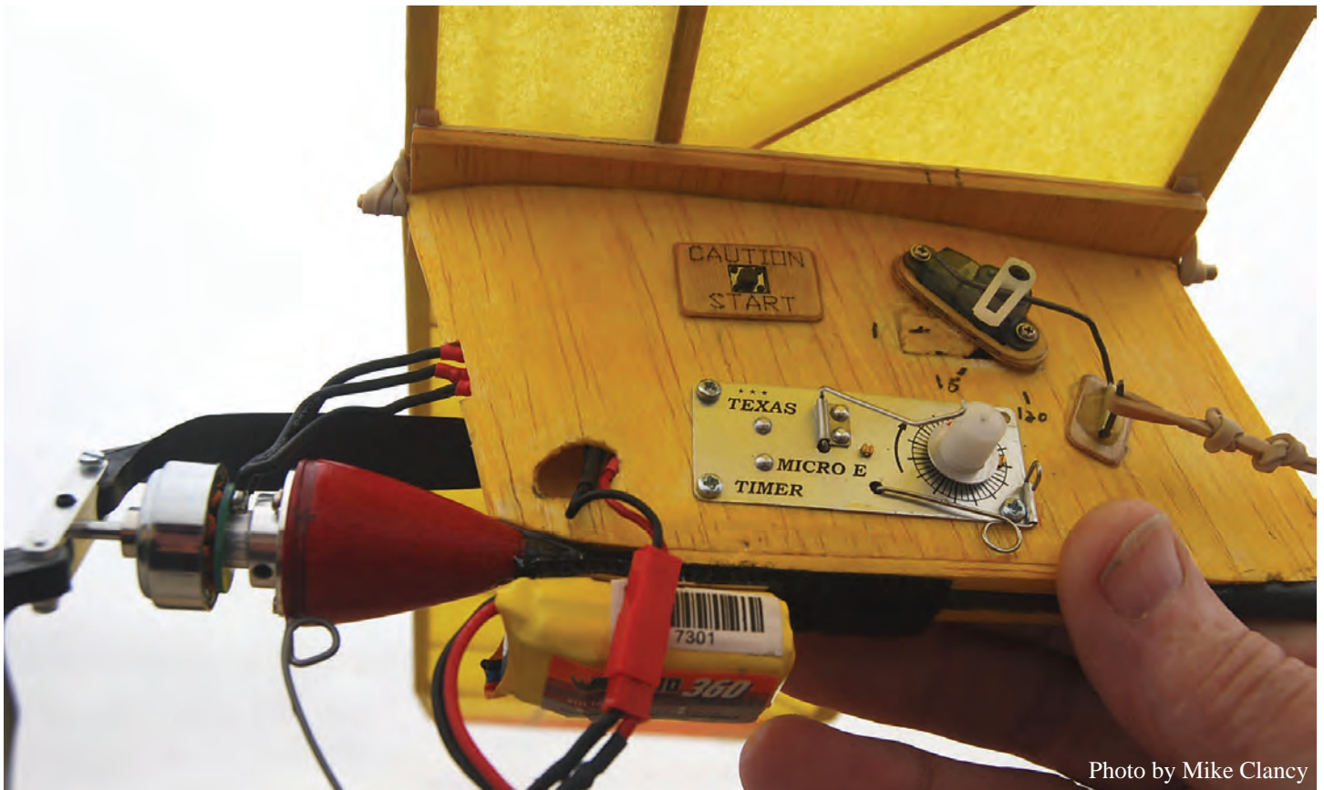
Dick Irwin's electric free flight showing folding prop, motor, battery, motor timer, dethermalizer timer, activator switch, etc. ...and free flight used to be so simple.
