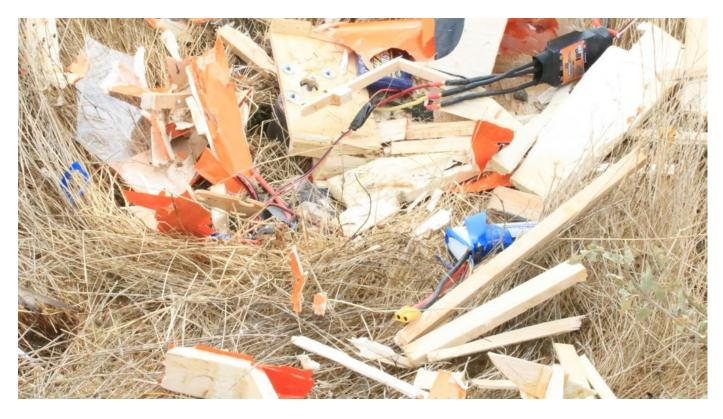
This is all that is left of the booster stage. It looks like another project to repair this one. What happened was that the front of the wing came up a slight bit and the force lifted it up and off of the fuselage. Breaking all tie-downs.
