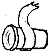
3. Drill hole in bottom for 4-40 screw after cutting to chosen size. Smooth up sawn top edge with flat sanding block & 150-180 sandpaper.
