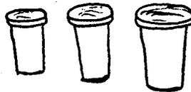
2. Mark cutting line by scoring in lathe or with masking tape. Use razor saw for final cut. Taper design will throw from lathe jaws if cut too deep.
